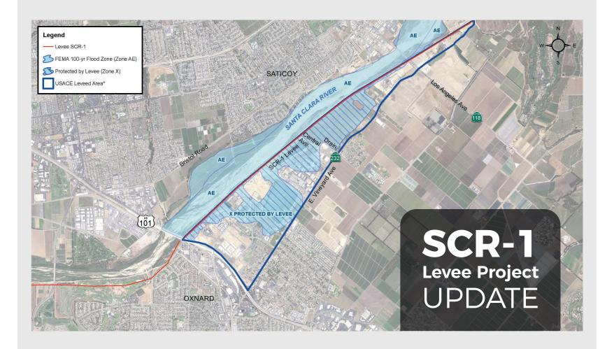
The SCR-1 levee, constructed in 1961 by the U.S. Army Corps of Engineers (USACE), and currently owned and maintained by the District, extends from Highway 101 to South Mountain along the east bank of the Santa Clara River. It provides flood protection to parts of the City of Oxnard, the Riverpark neighborhood, and unincorporated areas, including portions of the community of El Rio.
