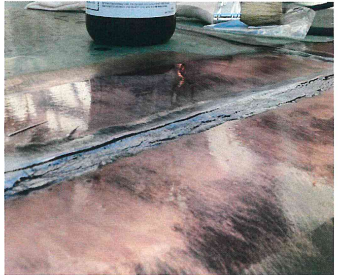
Metal substrates must be clean and primed with M-Prime.
