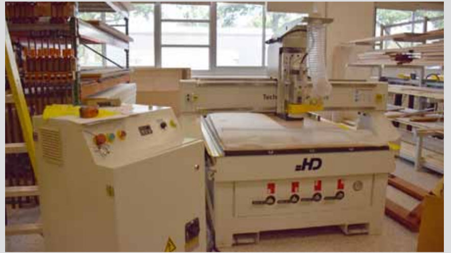
Pictured here, the CNC router makes cutting wood to precise measurements easier and safer for student use. It also allows for more elaborate works to be created.
