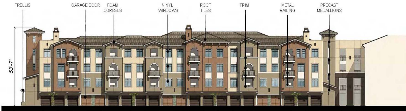
Building Type IV - Rear Elevation
