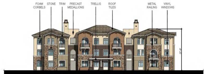
Building Type III - Front Elevation
