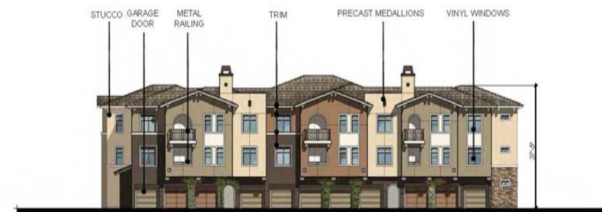
Building Type III - Rear Elevation
