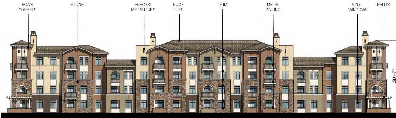
Building Type IV - Front Elevation Beach Boulevard
