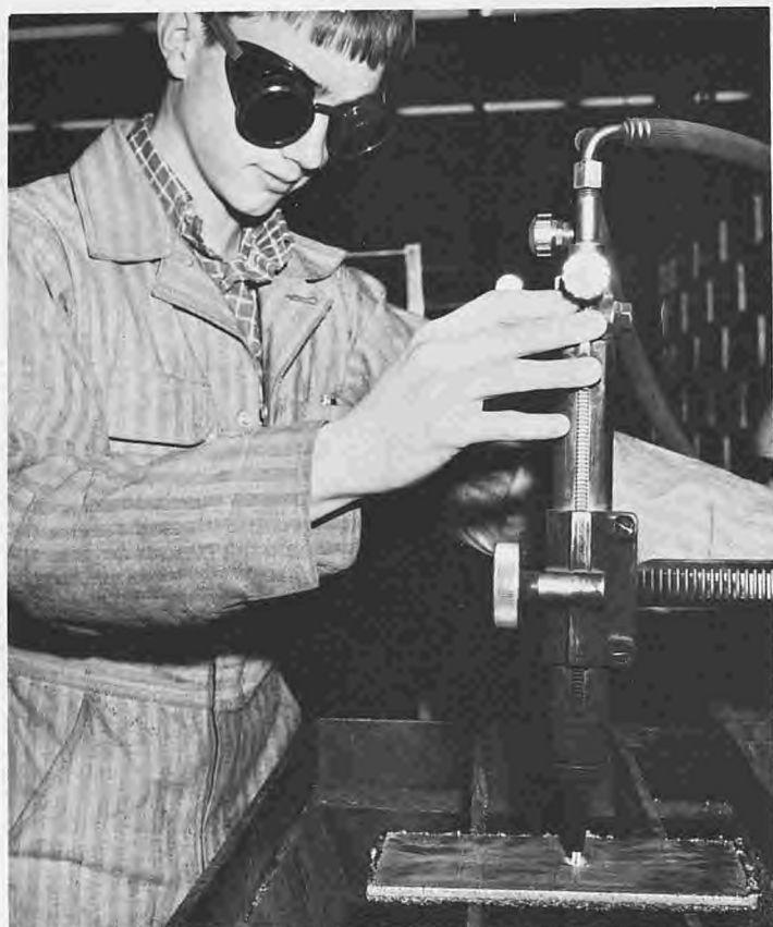
Using an automatic torch, Paul Cardon cuts a sheet of metal in general metals.
