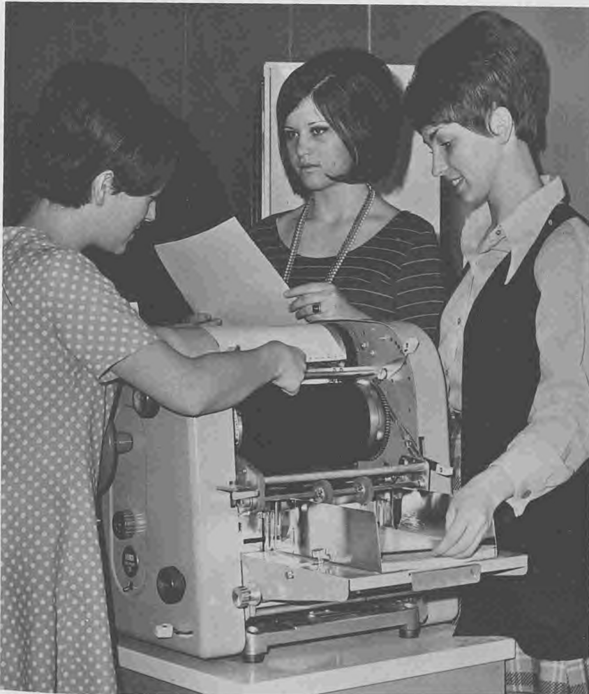
Clara Bell Ellett demonstrates attaching offset mat to the offset, a duplicating machine that gives the best reproduction possible, to Dorcus Maughan and KennaRae Munk.
