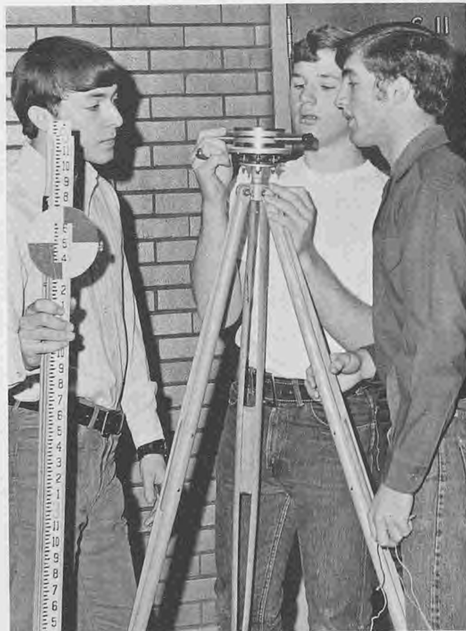
Dennis Cartwright, Michael Preece, and Val White determine the length of the hall by using a transit and trigonometry in Survey Math.
