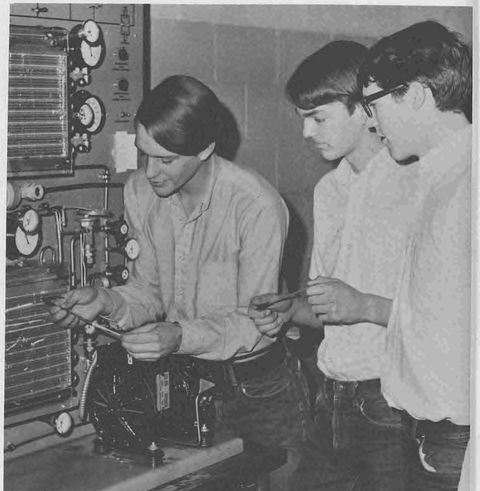
Clair Allen, Jeff Elwood, and Brad Johnson practice testing and checking out various types of freons in a model of a refrigerator-freezer in their two-hour block class Refrigeration and Air Conditioning.
