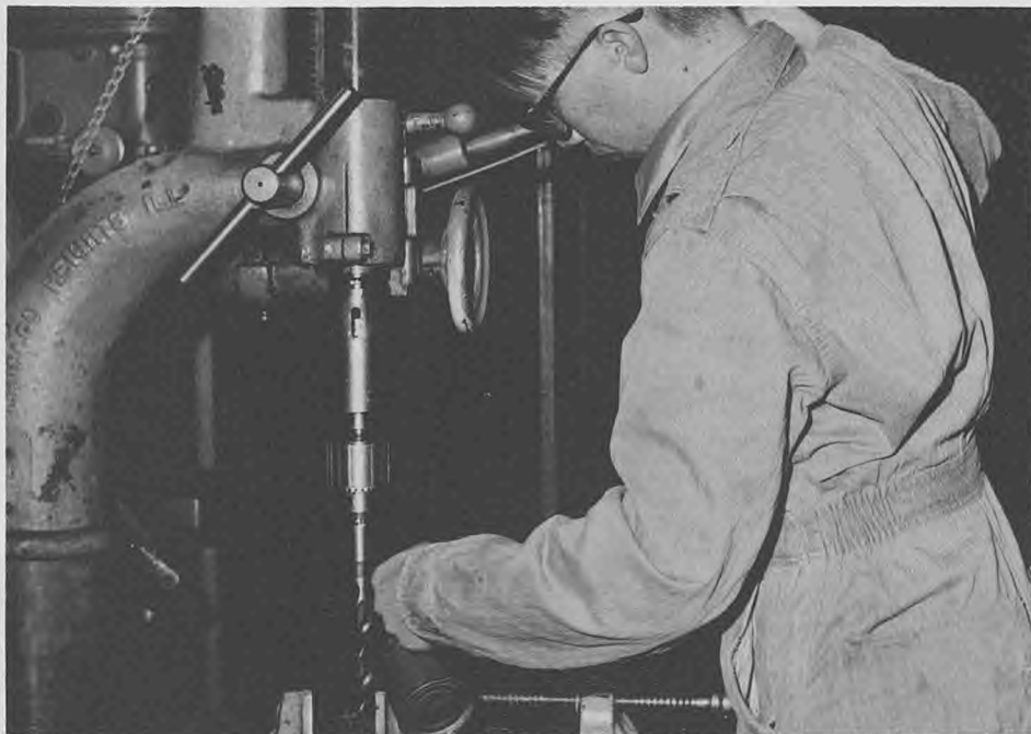
In his Agricultural Mechanics II class Clark Israelson adds oil so that his drill bit will not over heat while making a turntable that will pick up pigs and turn them over so he can trim their hooves.
