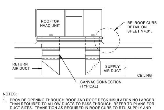
1. DRYWALL, METAL STUDS OR ANY OTHER RIGID MATERIAL MUST NOT TOUCH DUCT.
