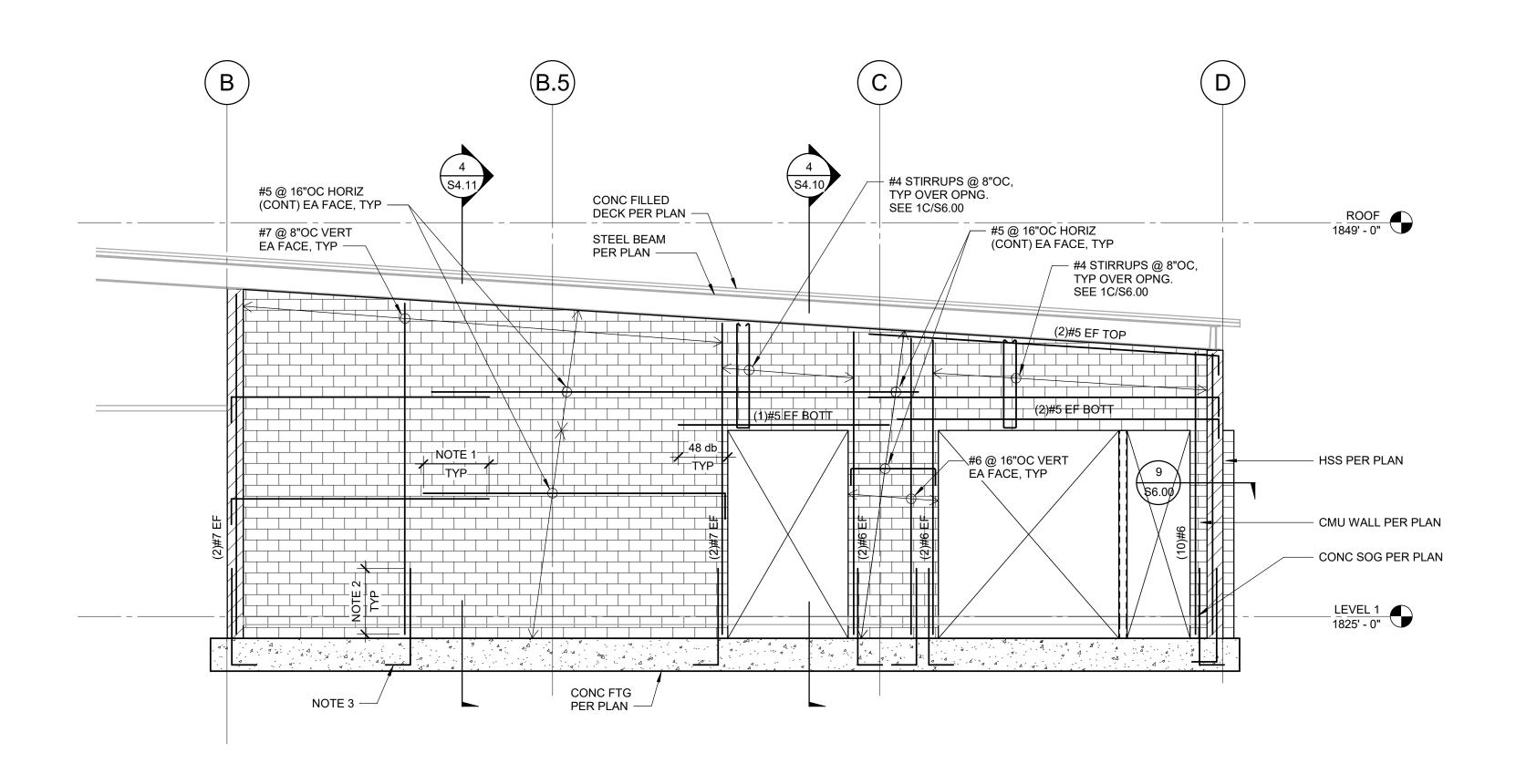
NOTES: 1. LAP SPLICE PER 4/S6.00. 2. LAP SPLICE PER 4/S6.00. 3. VERTICAL DOWELS TO MATCH SIZE AND SPACING OF CMU VERTICAL REINFORCING BARS.
