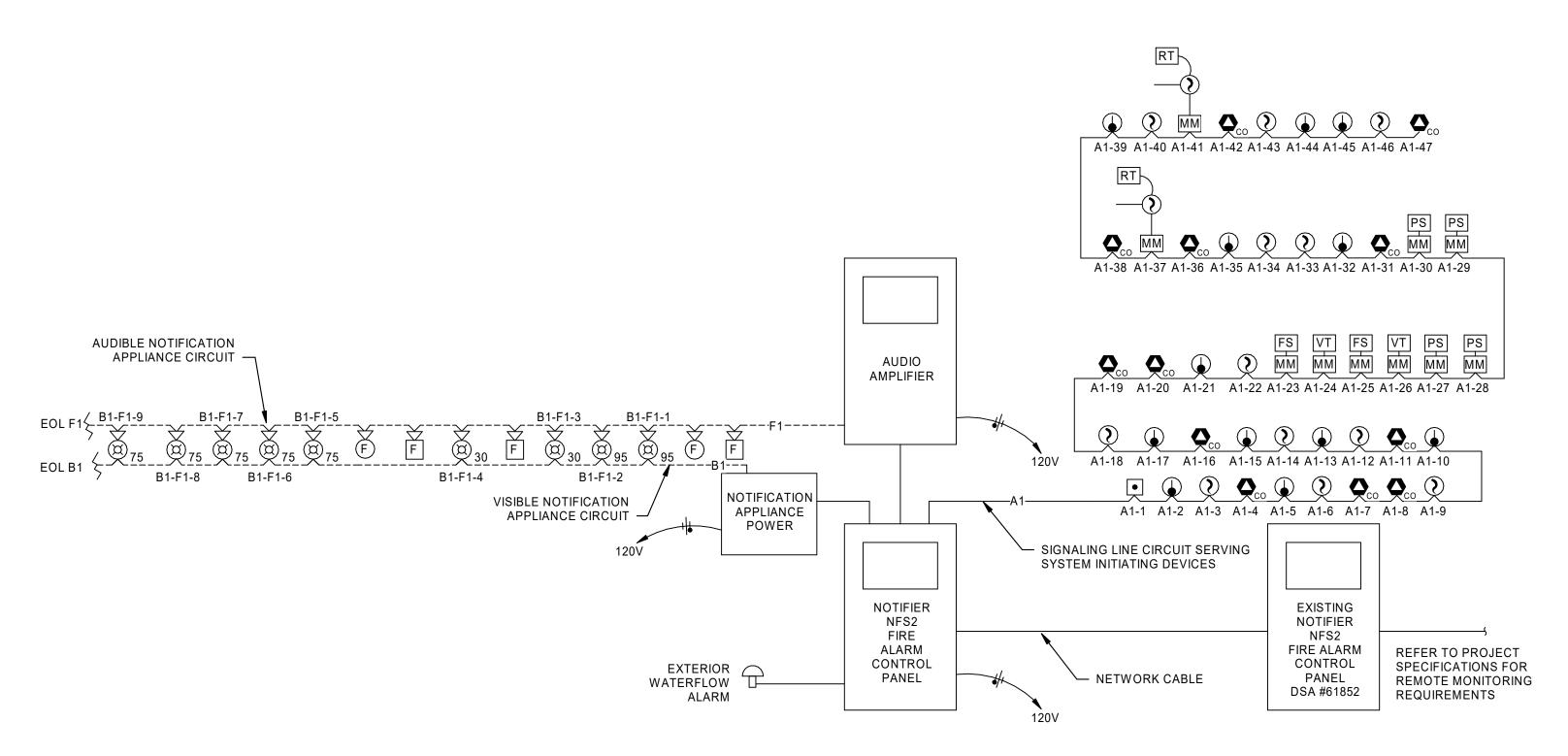
1 FIRE ALARM RISER DIAGRAM - ADDRESSABLE SYSTEM (VOICE) NTS
