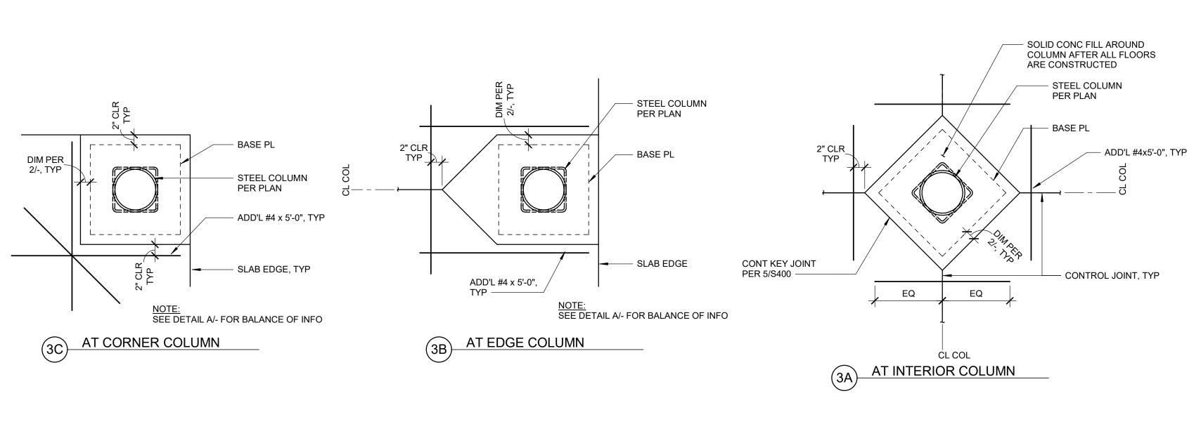
STEEL COLUMN BLOCK-OUT AT SLAB-ON-GRADE 3 SCALE : 1" = 1'-0"
