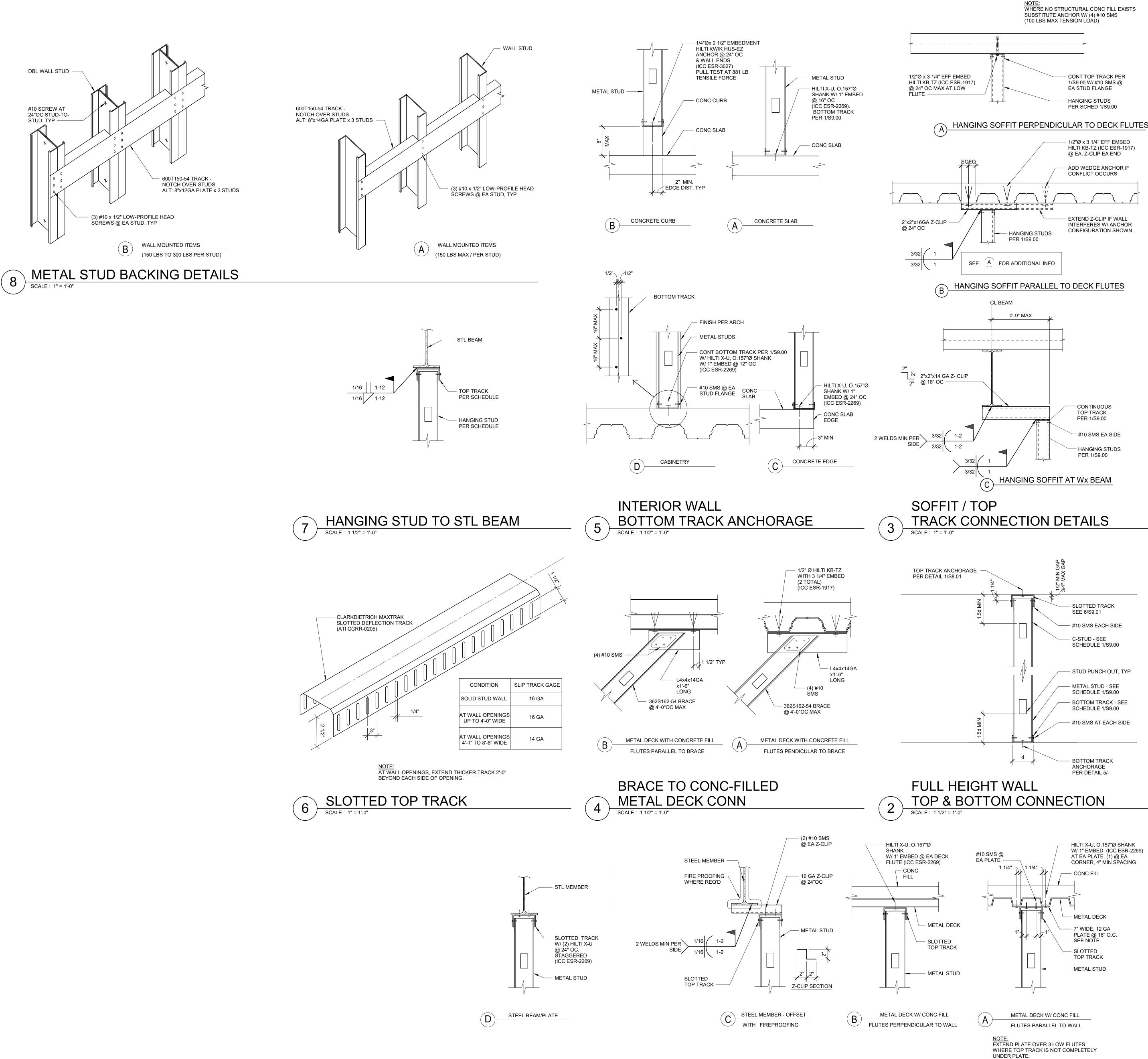
INTERIOR WALL TOP DEFLECTION/SLIP TRACK ANCHORAGE SCALE : 1 1/2" = 1'-0"
