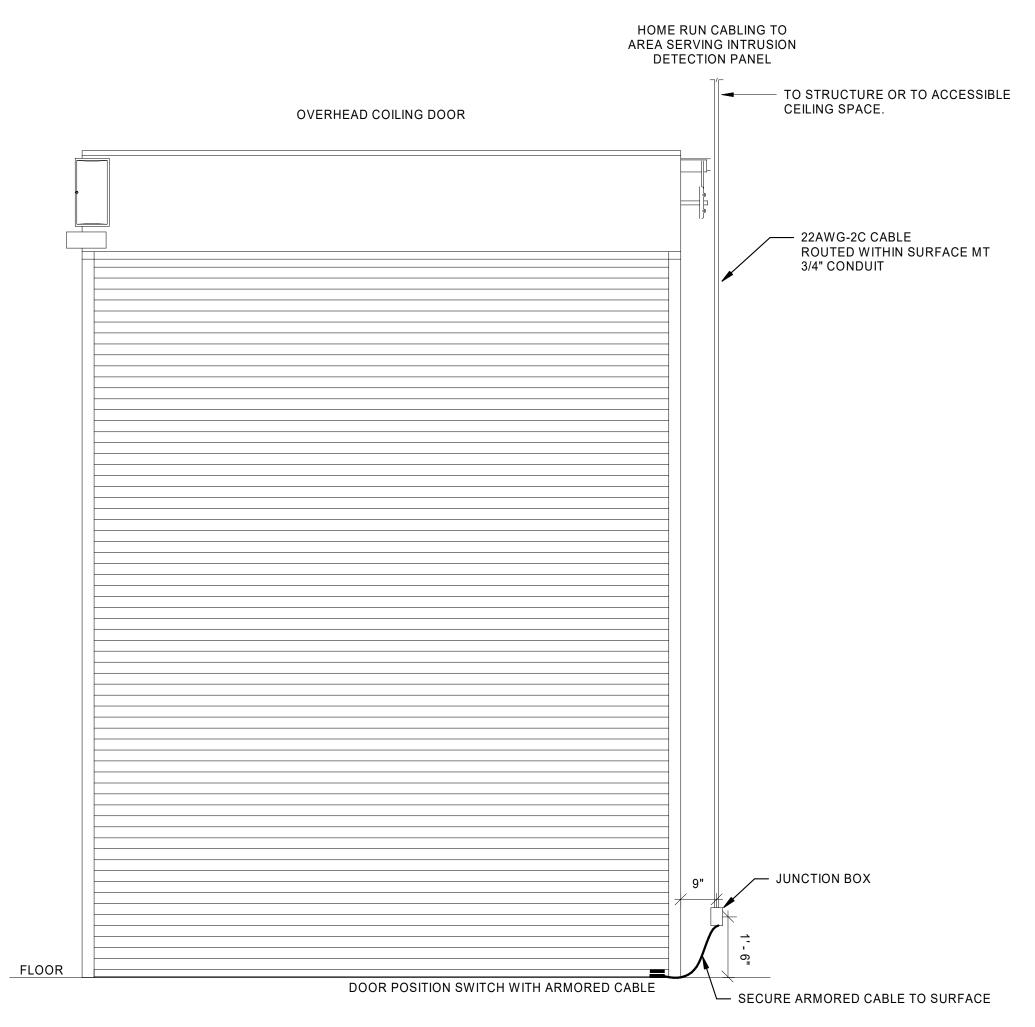
OVERHEAD COILING DOOR WITH FLOOR MOUNTED DOOR POSITION SWITCH NTS
