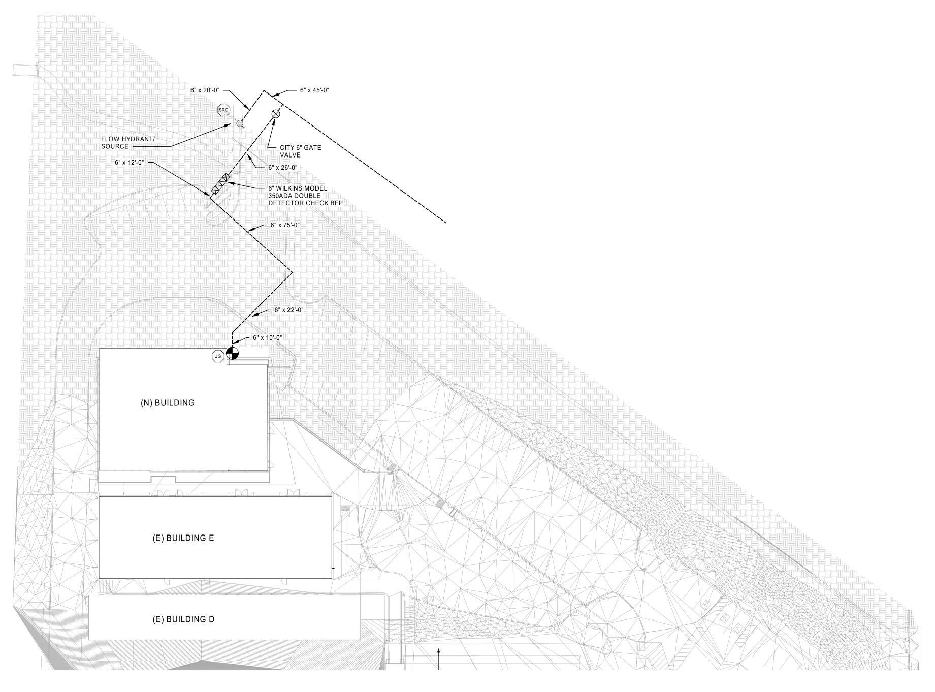
1 FIRE SPRINKLER SITE PLAN NTS FOR REFERENCE ONLY, SEE CIVIL ENGINEERING PLANS FOR FINAL LOCATIONS
