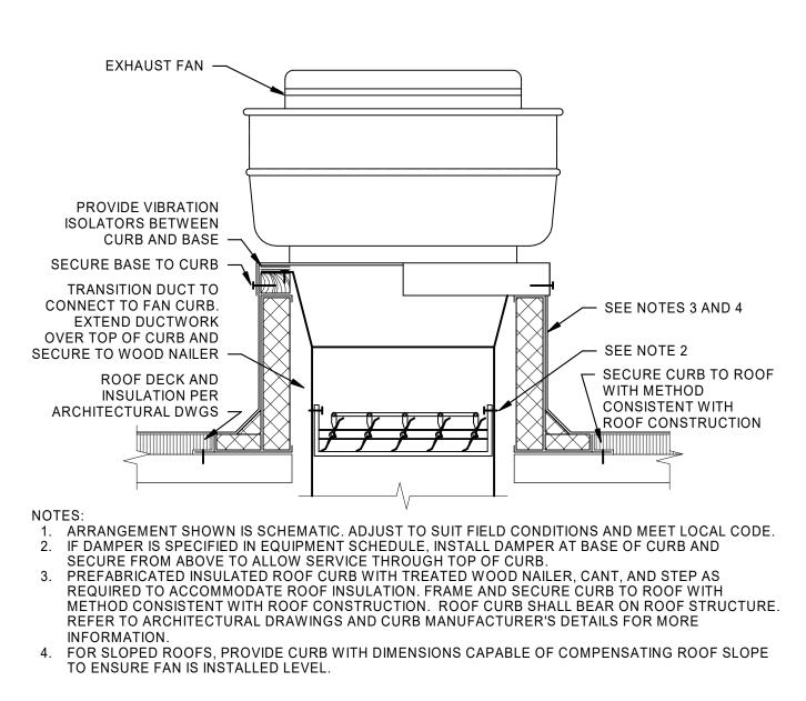
ROOF MOUNTED UPBLAST FAN DETAIL NTS
