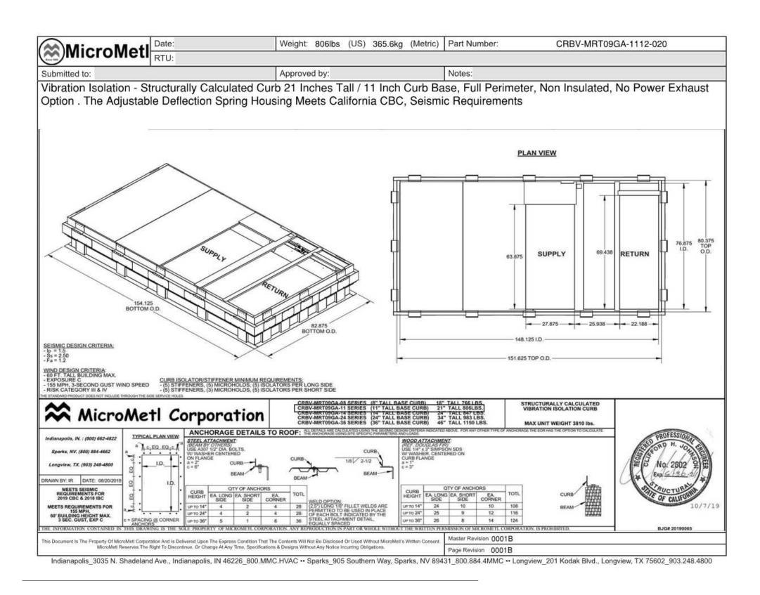
3 ROOFTOP UNIT VIBRATION ISOLATION DETAIL - RTU 1-2 NTS
