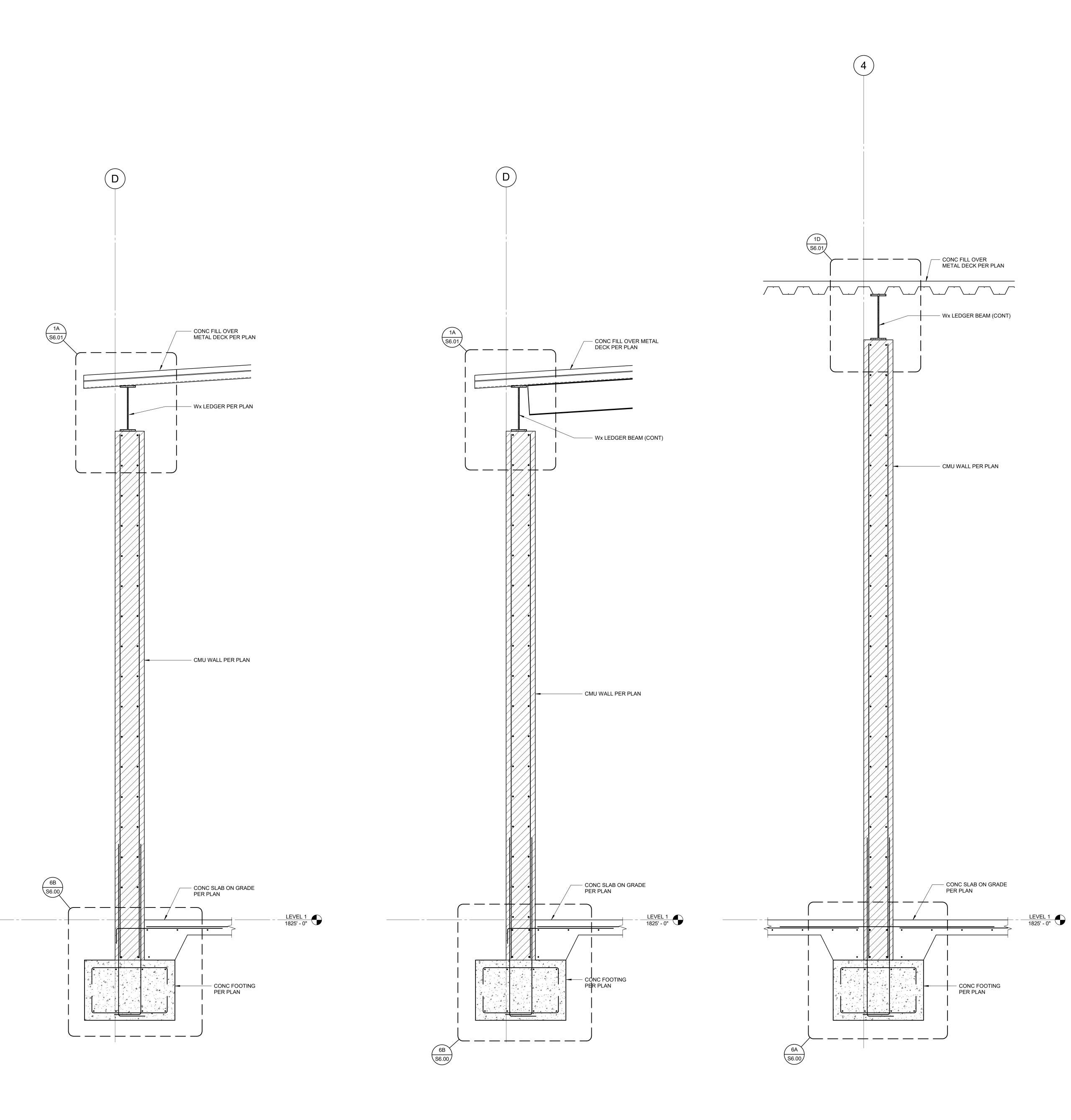
3 SECTION ALONG GRID D SCALE : 3/4" = 1'-0"
