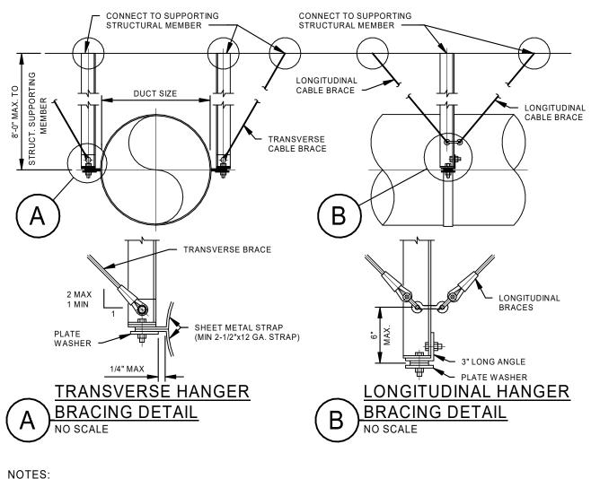
REFER TO STRUCTURAL SHEET S8.00 FOR ATTACHMENT TO STRUCTURE..
