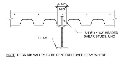
POSSIBLE OR DECK MUST BE SPLIT FULL LENGTH OF BEAM TO PROVIDE CONCRETE HAUNCH WITH MIN. WIDTH OF 4 1/2". SEE 6/- FOR MORE INFO.
