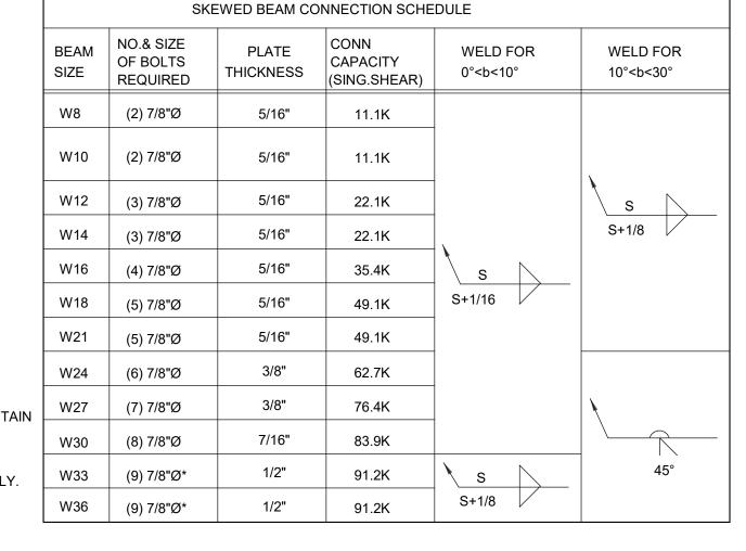
3. DO NOT INCREASE DIM X WITHOUT ENGINEER'S APPROVAL. 4. \* USE HORIZ SHORT SLOTTED HOLES IN PLATE AT COL CONN ONLY.
