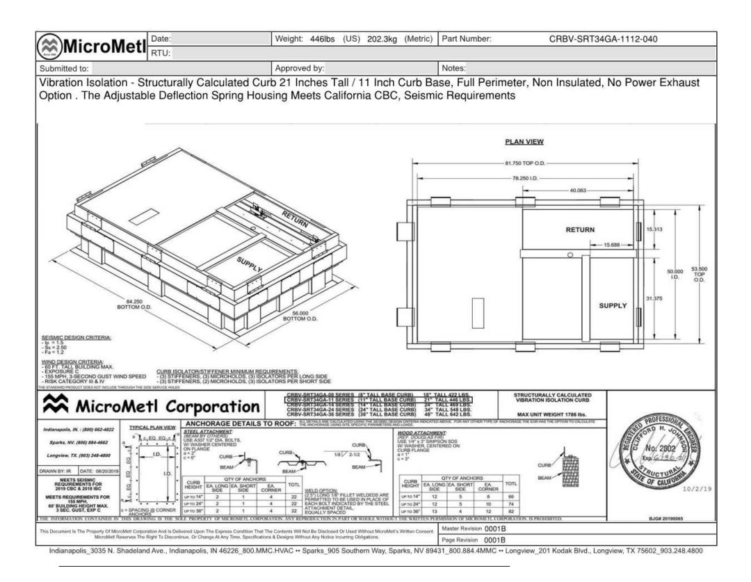
ROOFTOP UNIT VIBRATION ISOLATION DETAIL - RTU 1-1
