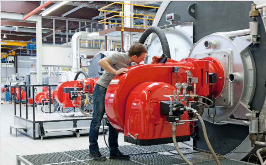
Test-firing chambers for medium and large-sized burners at the Weishaupt Research & Development Centre
