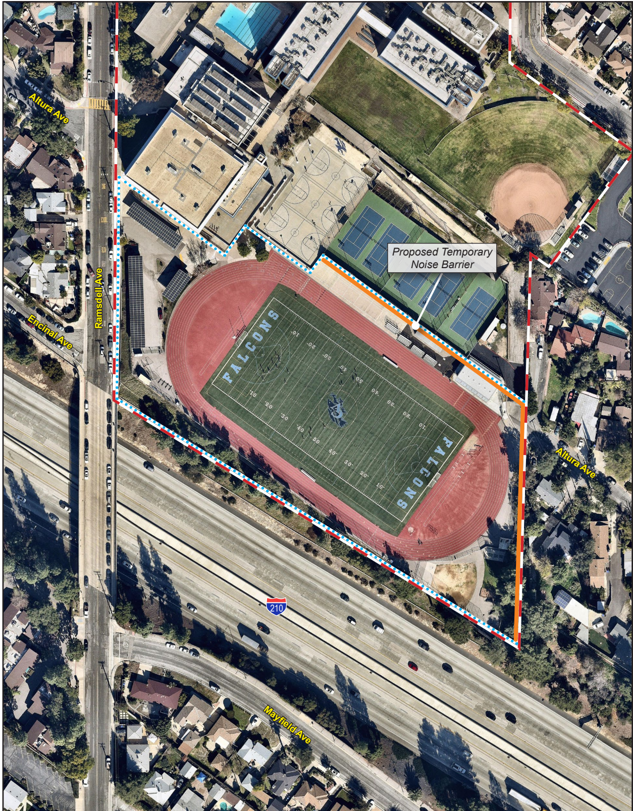
Figure 5.8-3 - Proposed Temporary Noise Barrier 5. Environmental Analysis
