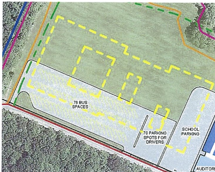
Space required for bus and driver parking, shown relative to existing Fuller building footprint
