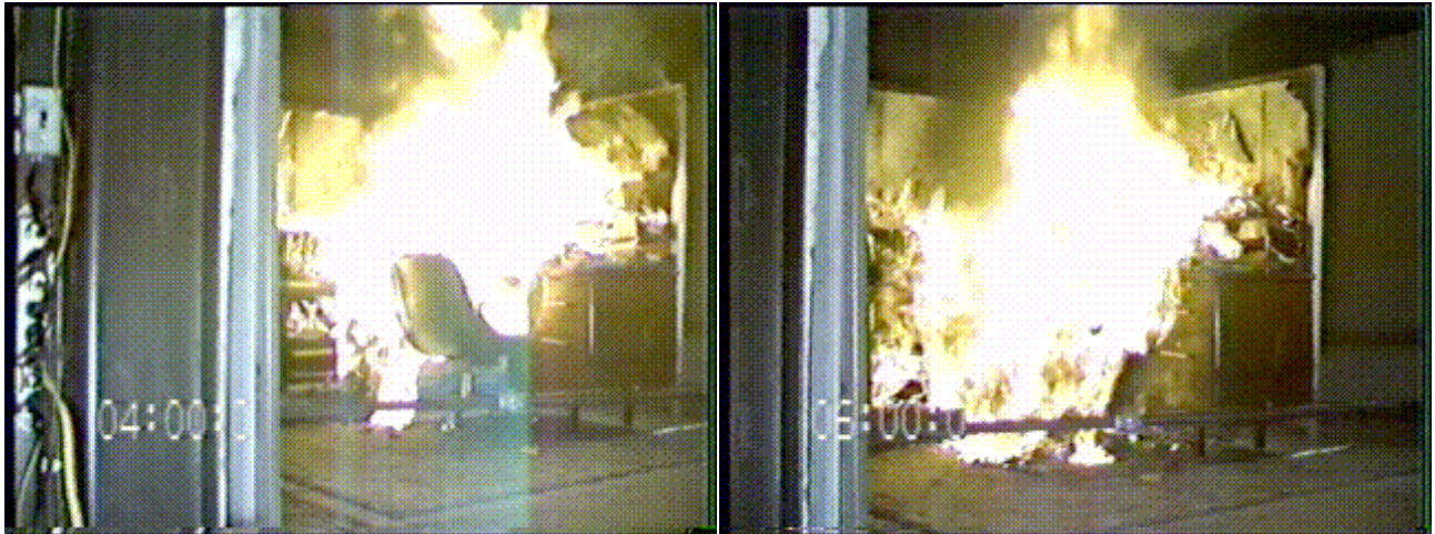
Figure 45: Two Panel Workstation fire at time 4:00 and 6:00 minutes
