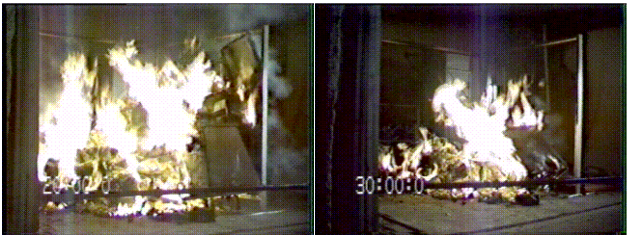
Figure 47: Two Panel Workstation fire at time 20:00 and 30:00 minutes
