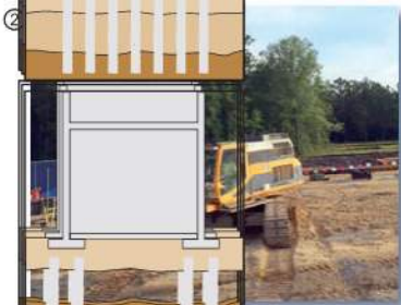
① RIs to support future fill and building loads for a grocery store.
