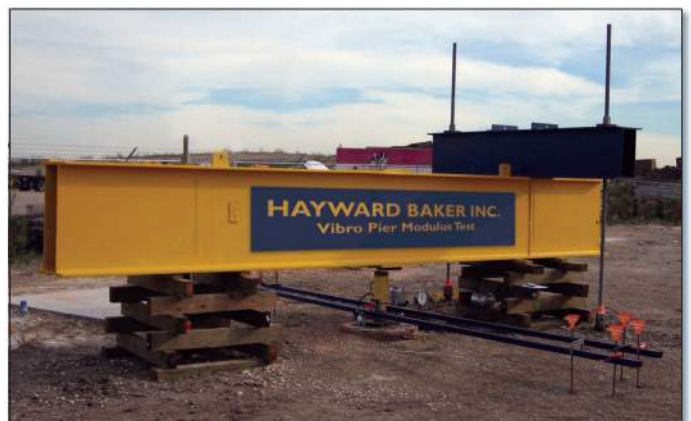
Vibro Pier Modulus Test to verify system performance.
