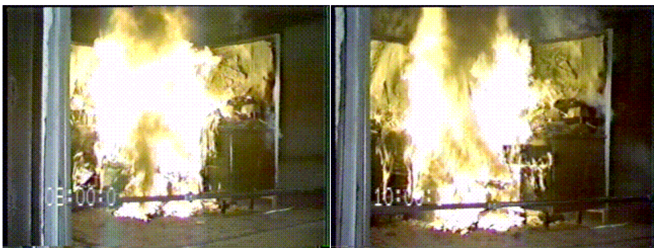
Figure 46: Two Panel Workstation fire at time 8:00 and 10:00 minutes
