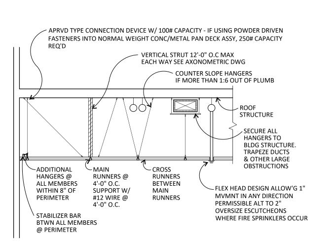
SUSPENDED CEILINGS SHALL BE FURNISHED AND INSTALLED PER CISCA STANDARDS AND THE ADDITIONAL REQUIREMENTS LISTED IN ASCE 7-10. UNLESS CEILING CLOUD DESIGN PROPOSED, SECURE GRID @ (2) SIDES MIN. TO WALLS OR HEADWALLS & INTERRUPT AREAS GREATER THAN 2,500 SQ FT W/ SEISMIC SEPARATION JT OR WALL/SOFFIT AS INDICATED IN PLANS. FOR CLOUD ASSY'S, PROVIDE ADD'L DESIGN DETAILING & ENGINEERING AS REQ'D BY AUTHORITIES HAVING JURISDICTION
