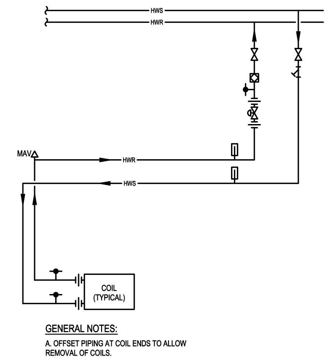
HEATING COIL PIPING DETAIL
