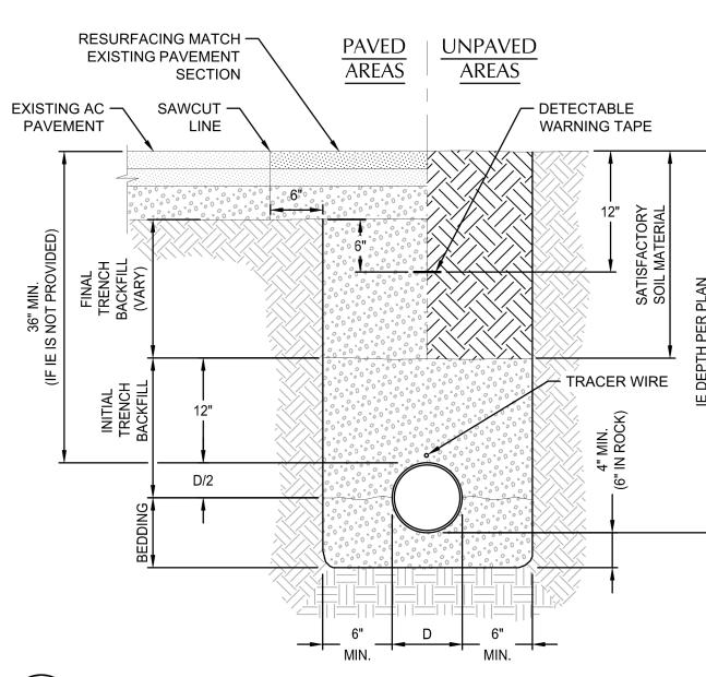
1 TYPICAL PIPE BEDDING AND BACKFILL
