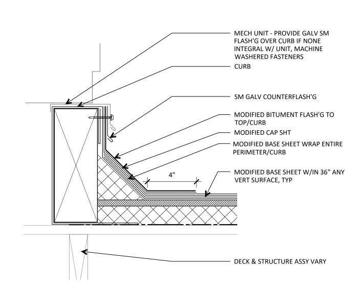
11 ROOF TOP MECHANICAL UNIT CURB, TYPICAL
