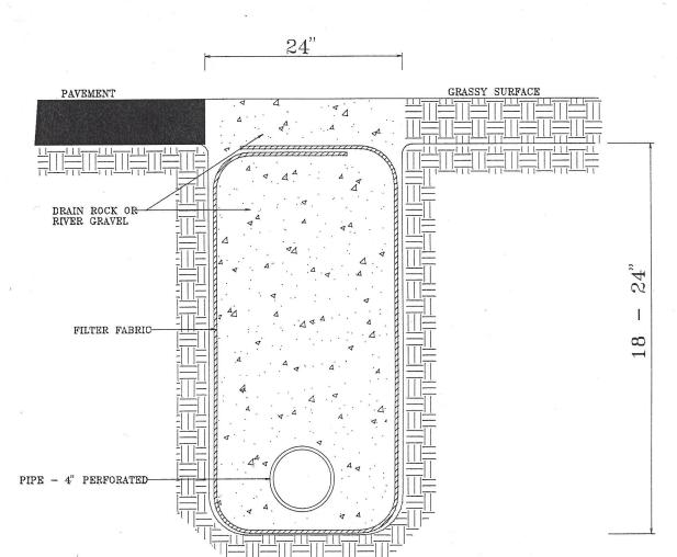
BRAUN INTERTEC TYPICAL FRENCH DRAIN STORMWATER DISPOSAL TRENCH DRAWN BY: JCU
