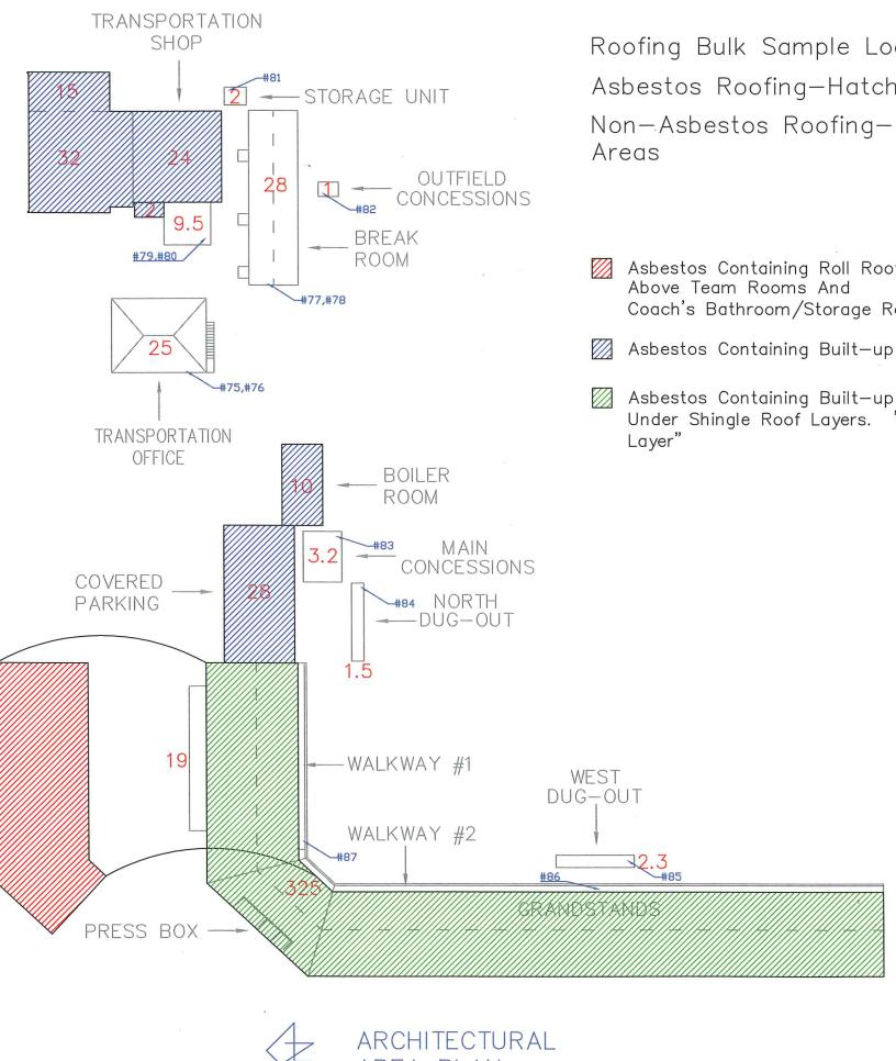
Roofing Bulk Sample Locations Asbestos Roofing-Hatched Areas Non-Asbestos Roofing-Unhatched
