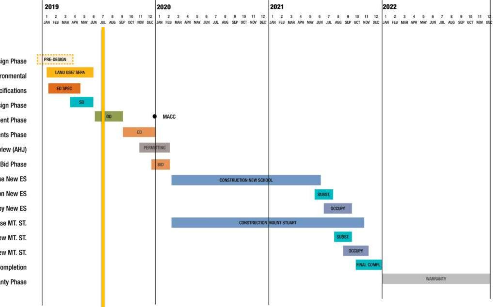
**Predesign Phase** Land Use/Evironmental **Educational Specifications** Schematic Design Phase **Design Development Phase Construction Documents Phase** Permit Document Review (AHJ) **Bid Package/ Bid Phase Construction Phase New ES** Substantial Completion New ES Occupy New ES Construction Phase MT. ST. Substantial Completion New MT. ST. Occupy New MT. ST. **Final Completion** Warranty Phase
