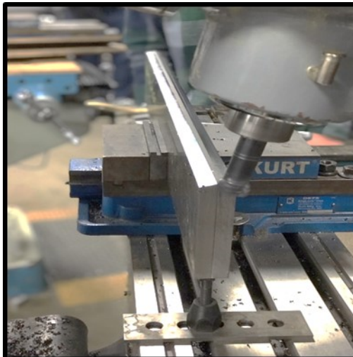
Fabrication of new blade with stronger metal
