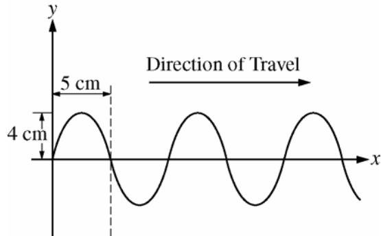
The figure above shows a transverse wave traveling to the right at a particular instant of time. The period of the wave is  $0.2 \text{ s}$ .
