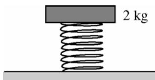
60. A platform of mass 2 kg is supported by a spring of negligible mass as shown above. The platform oscillates with a period of 3 s when the platform is pushed down and released. What must be the mass of a block that when placed on the platform doubles the period of oscillation to 6 s?
