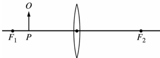
An object  $O$  is located at point  $P$  to the left of a converging lens, as shown in the figure above.  $F_1$  and  $F_2$  are the focal points of the lens.
