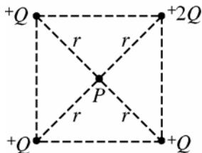
Four positive charges are fixed at the corners of a square, as shown above. Three of the charges have magnitude  $Q$ , and the fourth charge has a magnitude  $2Q$ . Point  $P$  is at the center of the square at a distance  $r$  from each charge.
