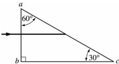
56. A ray of light in air is incident on a  $30^\circ$ - $60^\circ$ - $90^\circ$  prism, perpendicular to face  $ab$ , as shown in the diagram above. The ray enters the prism and strikes face  $ac$  at the critical angle. What is the index of refraction of the prism?
