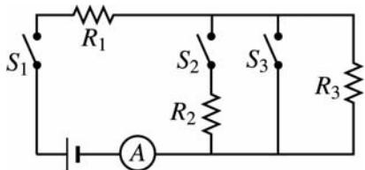
In the circuit above, the resistors all have the same resistance. The battery, wires, and ammeter have negligible resistance. A closed switch also has negligible resistance.
