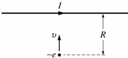
An electron of charge  $-e$  and a long straight wire carrying a current  $I$  to the right are both in the plane of the page, as shown above. In the position shown, the electron is a distance  $R$  from the wire and is moving directly toward it with speed  $v$ .
