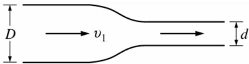
18. Water flows through the pipe shown above. At the larger end, the pipe has diameter  $D$  and the speed of the water is  $v_1$ . What is the speed of the water at the smaller end, where the pipe has diameter  $d$ ?
