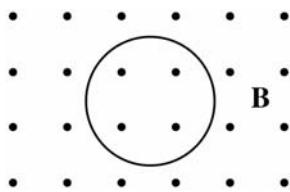
33. A uniform magnetic field  $\mathbf{B}$  is directed out of the page, as shown above. A loop of wire of area  $0.40 \text{ m}^2$  is in the plane of the page. At a certain instant the field has a magnitude of  $3.0 \text{ T}$  and is decreasing at the rate of  $0.50 \text{ T/s}$ . The magnitude of the induced emf in the wire loop at this instant is most nearly
