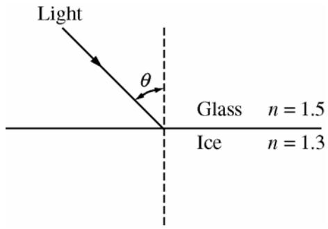
39. A ray of light in glass that is incident on an interface with ice, as shown above, is partially reflected and partially refracted. The index of refraction  $n$  for each of the two media is given in the figure. How do the angle of reflection and the angle of refraction compare with the angle of incidence  $\theta$ ?
