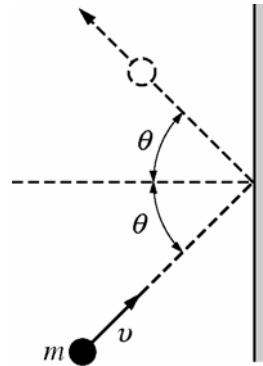
66. A ball of mass  $m$  with speed  $v$  strikes a wall at an angle  $\theta$  with the normal, as shown above. It then rebounds with the same speed and at the same angle. The impulse delivered by the ball to the wall is
