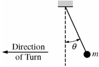
70. An object of mass  $m$  hangs from a string that is fixed to the ceiling of a car. At the instant shown above, the car is moving into the plane of the page at constant speed  $v$  as it turns to the left around a horizontal curve of radius  $r$ . Which of the following is a correct expression for the angle  $\theta$  of the string with respect to the vertical?
