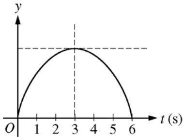
A ball is thrown straight up by a student at rest on the surface of Earth. A graph of the position  $y$  as a function of time  $t$ , in seconds, is shown above. Air resistance is negligible.
