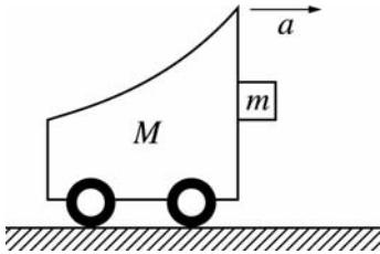
59. The figure above shows a cart of mass  $M$  accelerating to the right with a block of mass  $m$  held to the front surface only by friction. The coefficient of friction between the surfaces is  $\mu$ . What is the minimum acceleration  $a$  of the cart such that the block will not fall?
