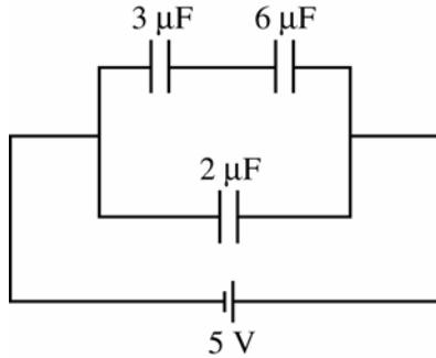
Three capacitors are connected to a 5 V source, as shown in the circuit diagram above.
