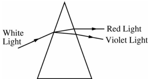
37. As shown above, a beam of white light is separated into separate colors when it passes through a glass prism. Red light is refracted through a smaller angle than violet light because red light has a
