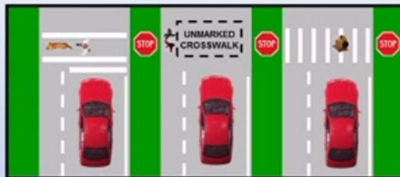
Stop lines and crosswalks
