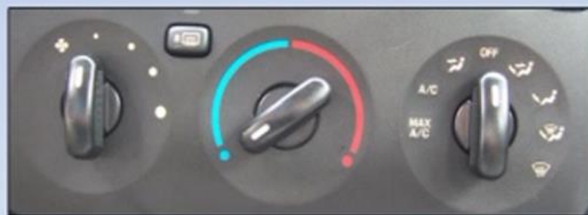
Heater, defroster, and air conditioner
