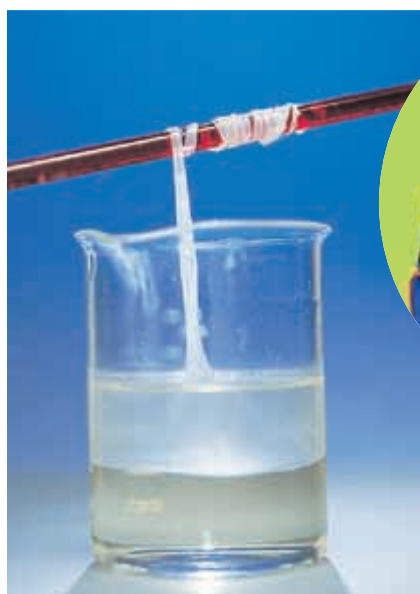
Figure 3 The white rope being pulled out of the liquid is nylon. Nylon forms at the surface between the two chemicals in the beaker. Nylon is one of the most widely used synthetic chemicals.
