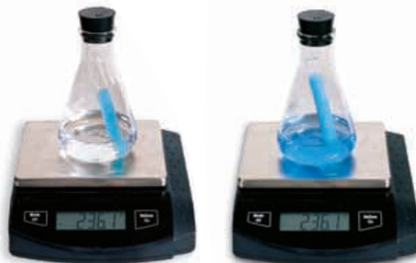
Figure 6 The total mass before the change is always the same as the total mass after the change.
