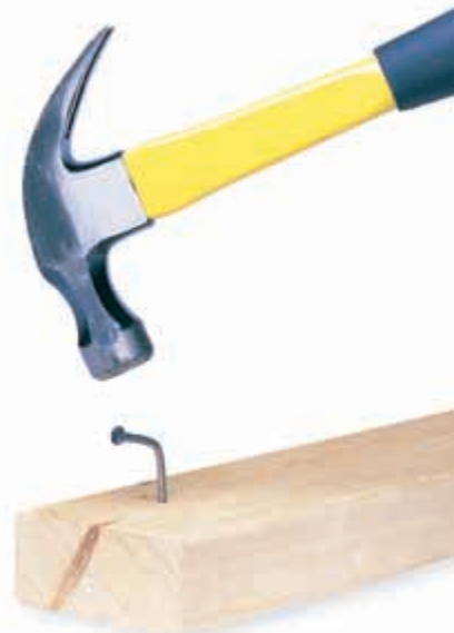
Figure 9 Metal can be reshaped without breaking because metallic bonds occur in many directions.
