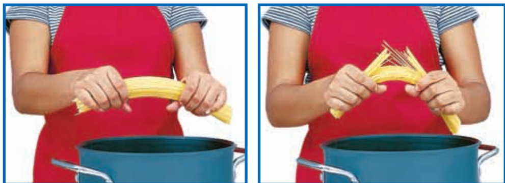
Figure 1 When a small amount of stress is placed on uncooked spaghetti, the spaghetti bends. Additional stress causes the spaghetti to break.
