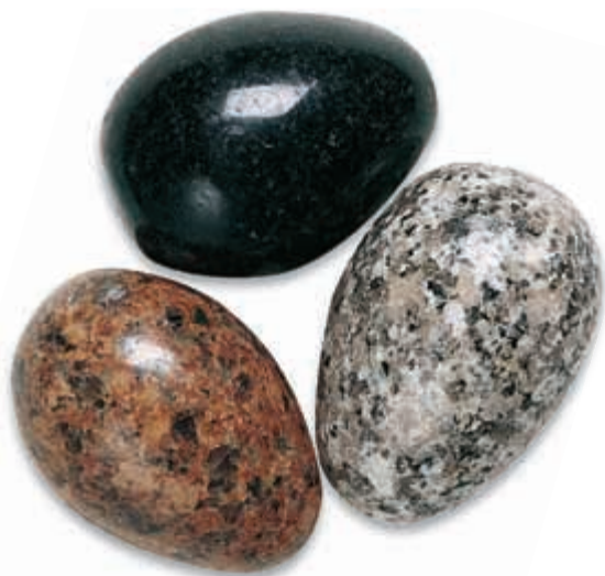
Figure 3 These paperweights are made of granite. They are different colors because the granite used in each has different ratios of minerals.
