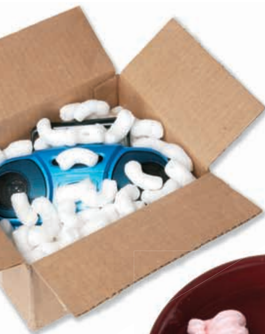
Figure 5 The radio is protected by starch-based peanuts. In just a few minutes, these peanuts dissolve in a bowl of water. The plastic-foam peanuts do not.
