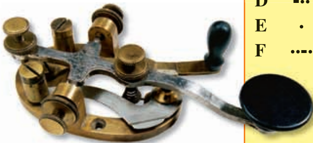
Figure 1 By tapping this telegraph key in the right combinations of short taps (dots) and long taps (dashes), people could send messages over long distances.
