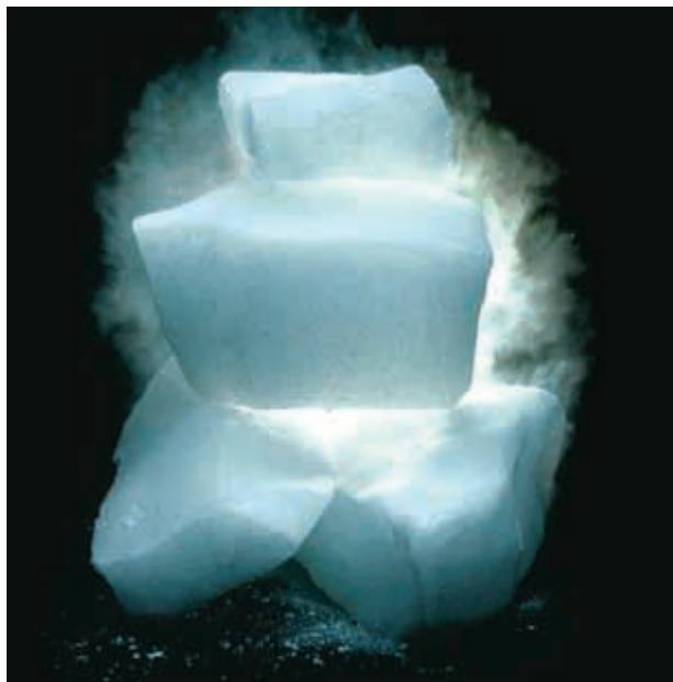
Figure 6 Dry ice changes directly from a solid to a gas. This change of state is called sublimation.
