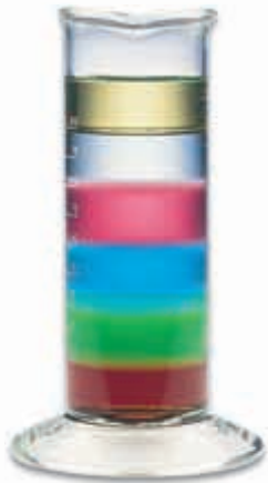
Figure 3 This graduated cylinder contains six liquids. From top to bottom, they are corn oil, water, shampoo, dish detergent, antifreeze, and maple syrup.
