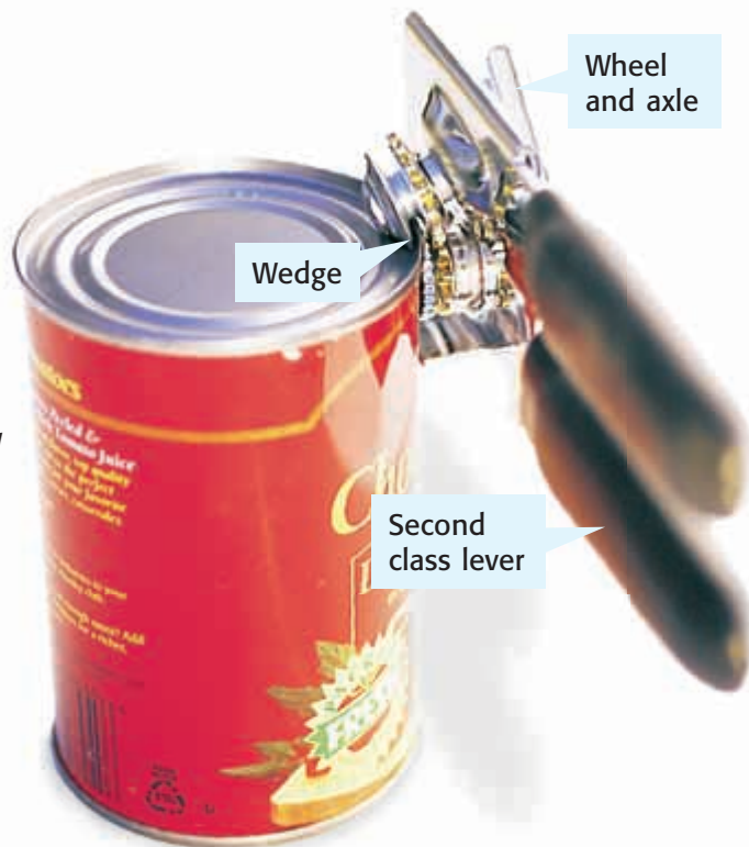
Figure 10 A can opener is a compound machine. The handle is a second-class lever, the knob is a wheel and axle, and a wedge is used to open the can.
