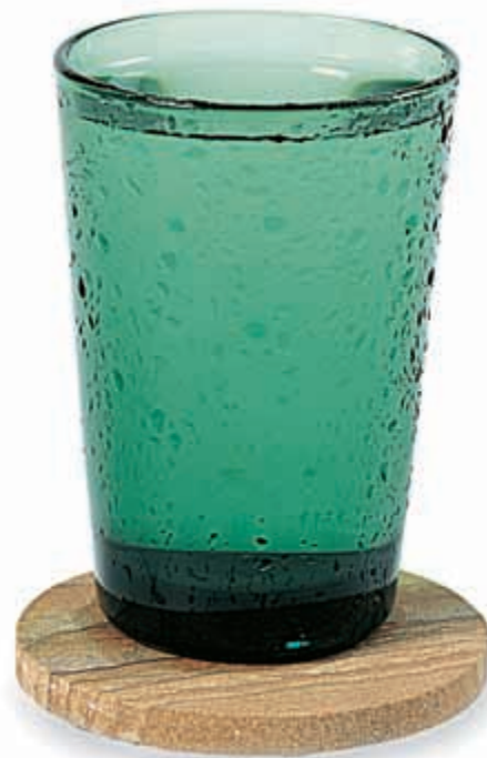
Figure 4 Condensation occurred when the air next to the glass cooled to its dew point.
