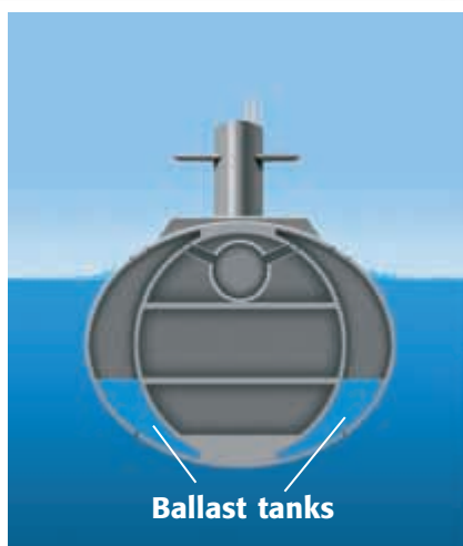
Figure 5 Controlling Density Using Ballast Tanks
