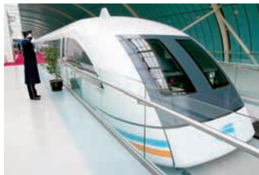
Figure 6 There is very little friction between this magnetic levitation train and its tracks, so it is highly efficient.
