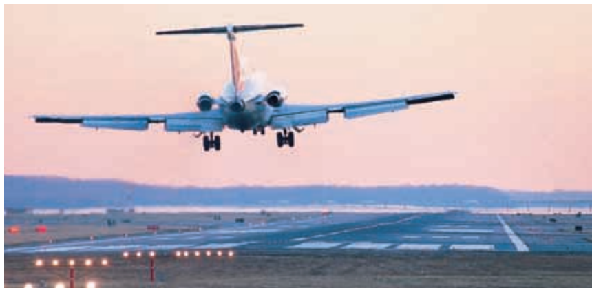
Figure 5 The pilot of this airplane can adjust these flaps to help increase lift when the airplane lands or takes off.
