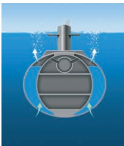
Figure 5 Controlling Density Using Ballast Tanks
