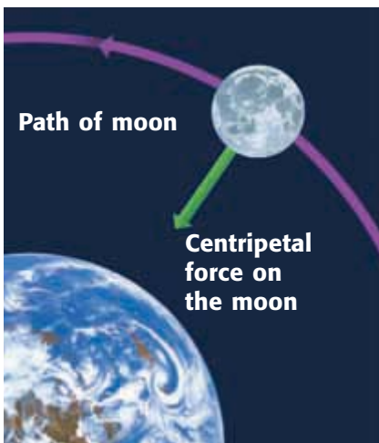
Figure 8 The moon stays in orbit around Earth because Earth's gravitational force provides a centripetal force on the moon.
