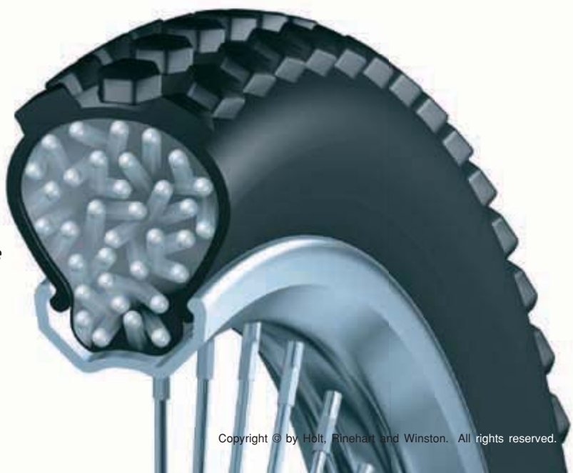
Figure 1 The force of the air particles hitting the inner surface of the tire creates pressure, which keeps the tire inflated.
