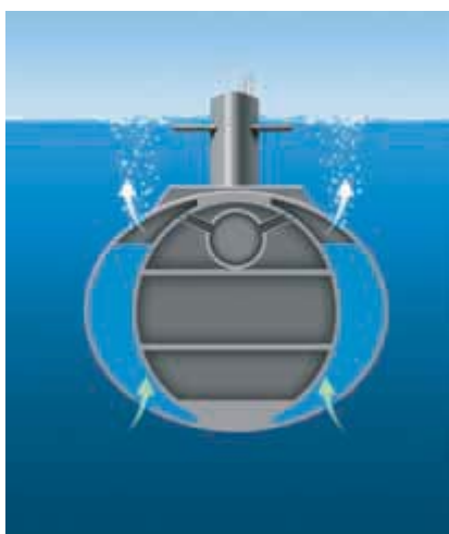
Figure 5 Controlling Density Using Ballast Tanks
