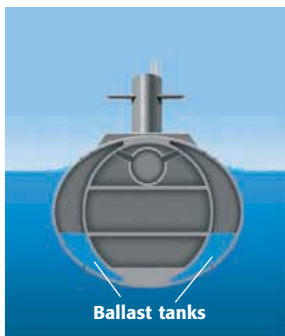
Figure 5 Controlling Density Using Ballast Tanks
