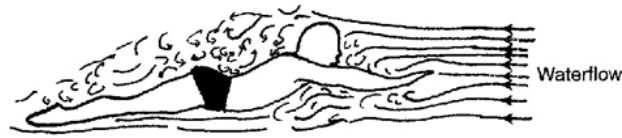
Large drag in unstreamlined position
