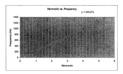
The slope of this graph, as shown by the equation, is (v/2L), and calculated by Microsoft Excel to be 243.27, meaning that (v/2L) = 243.27. With this information, and knowing that the length of our tube was 0.739 m, we can solve for the velocity:
