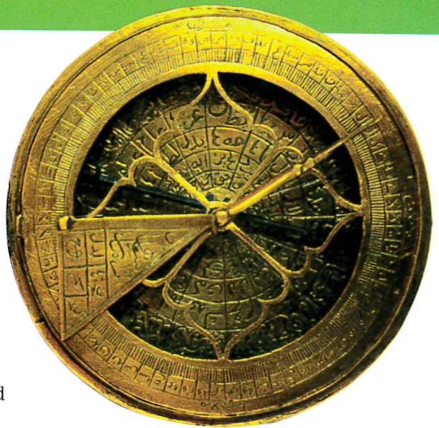
▲ The astrolabe helped sea captains determine the latitude of their ships.
