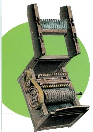
**Analyze Images** Workers fed cotton bolls through the gin's teeth and barbed roller to separate out the seeds and straighten the fibers. Using the gin, workers could produce much more cotton in a day. Predict Consequences How would this invention affect the demand for slaves?
